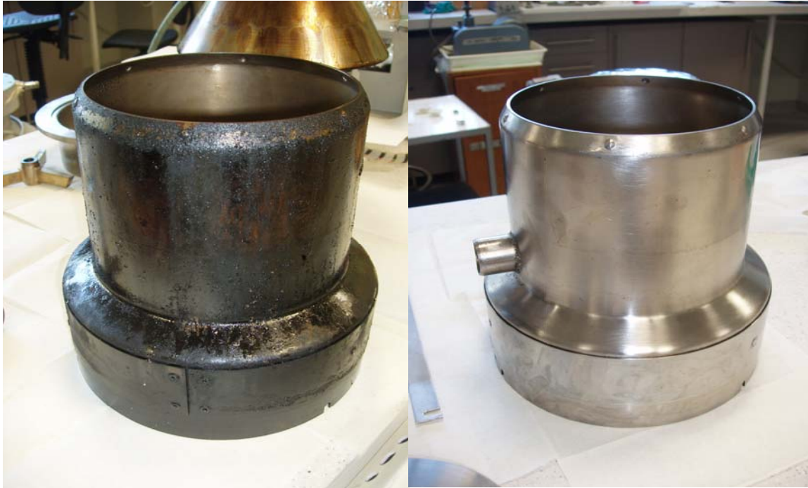
Figure 16 – Before and after comparison of internal component of DiffStak diffusion pump
