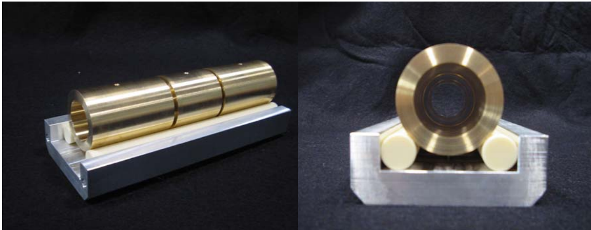
Figure 10- Einzel lens stack from side and front profile. Note the three segments and ceramic posts to electrically isolate the assembly
