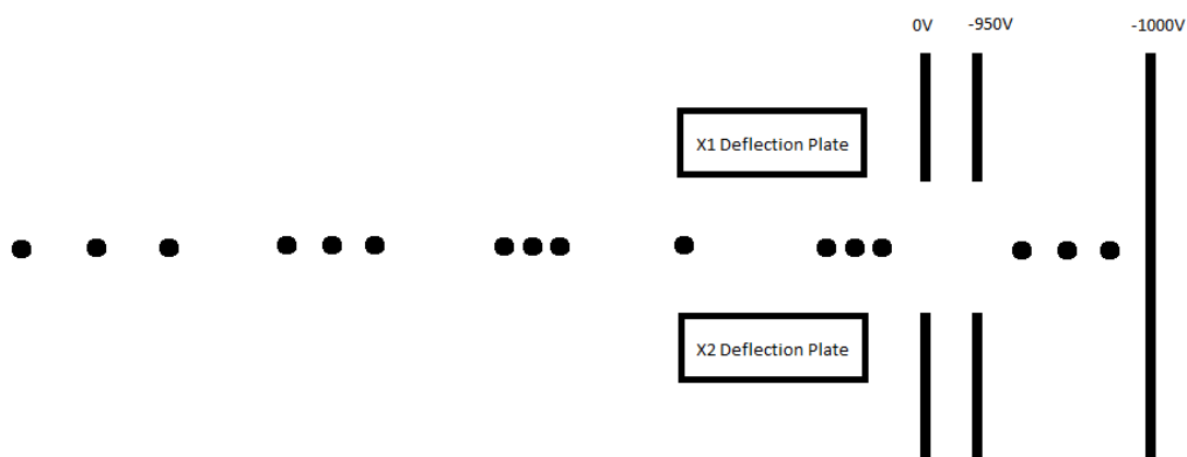
Figure 12 – An exaggerated example of spatial focussing with ions of the same mass starting at different distances from the back plate. After receiving different velocities they slowly group up until a ‘focal point’ (single point) is reached after which they spread out. The X deflection plates have been included and Y deflection plates are not in the same plane as the image. This diagram is not to scale.
